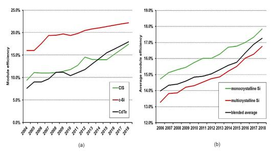
**Figure 2.** (a) Development in efficiency for the top products on the market. (b) Development of average efficiency in crystalline silicon modules [16].
