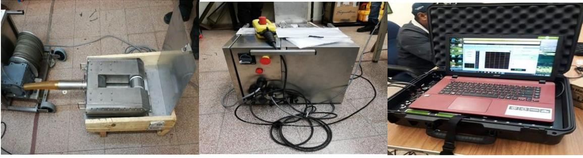
Fig. 2 The XDP30 and a winch (left), a control-command of the winch, and safety system for the generator of internal x-rays unit (center), and one computer with acquisition and control software (right).
