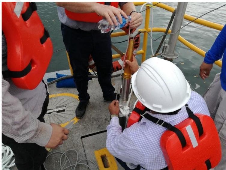
Fig. 7 Calibration of pressure sensor
