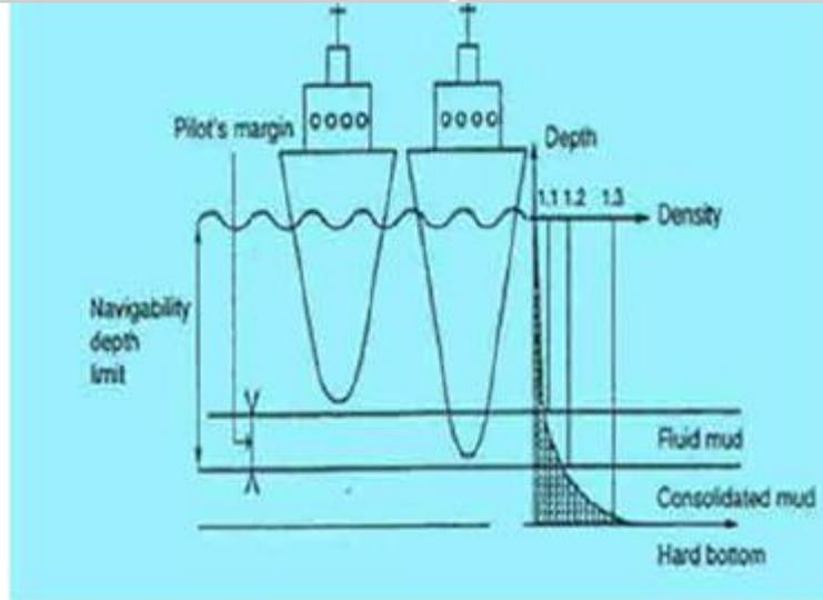
Fig. 10 Definition of the navigability depth limit in a sedimented channel. Image from [1]
