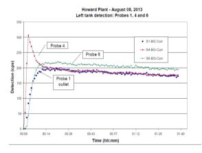
Fig. 7. Radiotracer detection in the left tank
