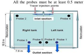
from any wall of the tanks just to avoid mechanical shocks that could damage the detector.
