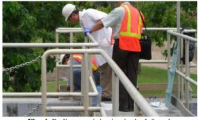
Fig. 4. Radiotracer injection in the left tank
